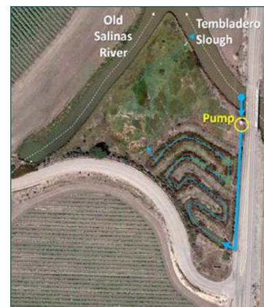
Molera Road wetland is an experimental off-line pollution treatment wetland.
